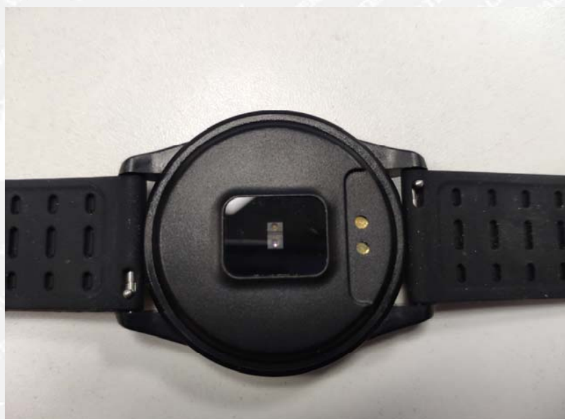
Photo 4 -- After the test of IPX7
