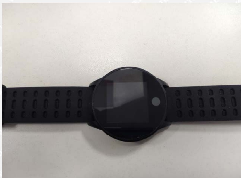
Photo 3 -- After the test of IPX7
