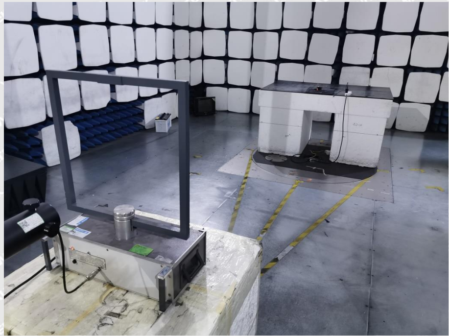
Radiated Spurious Emission Test Setup/ Radiated H-Field (Below 30MHz)
