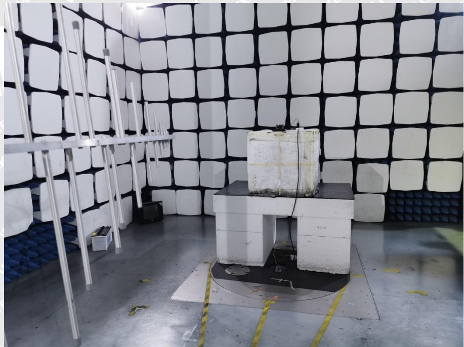
Radiated Spurious Emission Test Setup (Above 30MHz)
