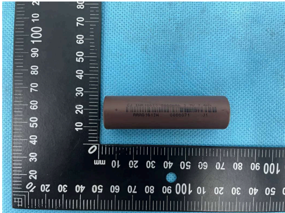
Figure 15 Front view of cell (Model: INR 18650-2000mAh)
