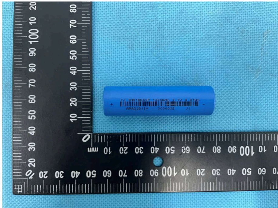
Figure 3 Front view of cell (Model: INR 18650P-1300mAh)
