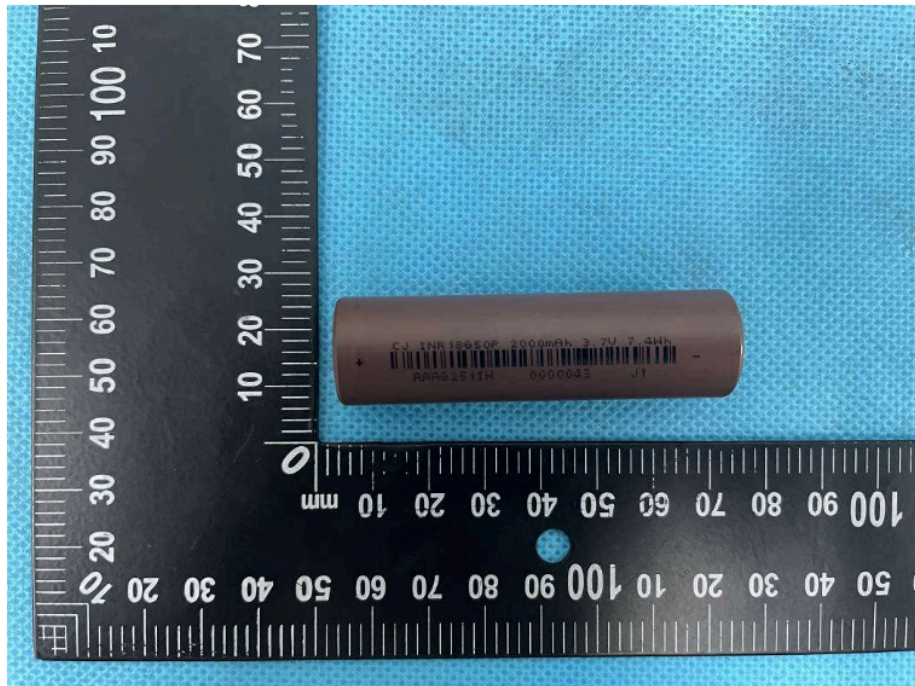
Figure 9 Front view of cell (Model: INR 18650P-2000mAh)
