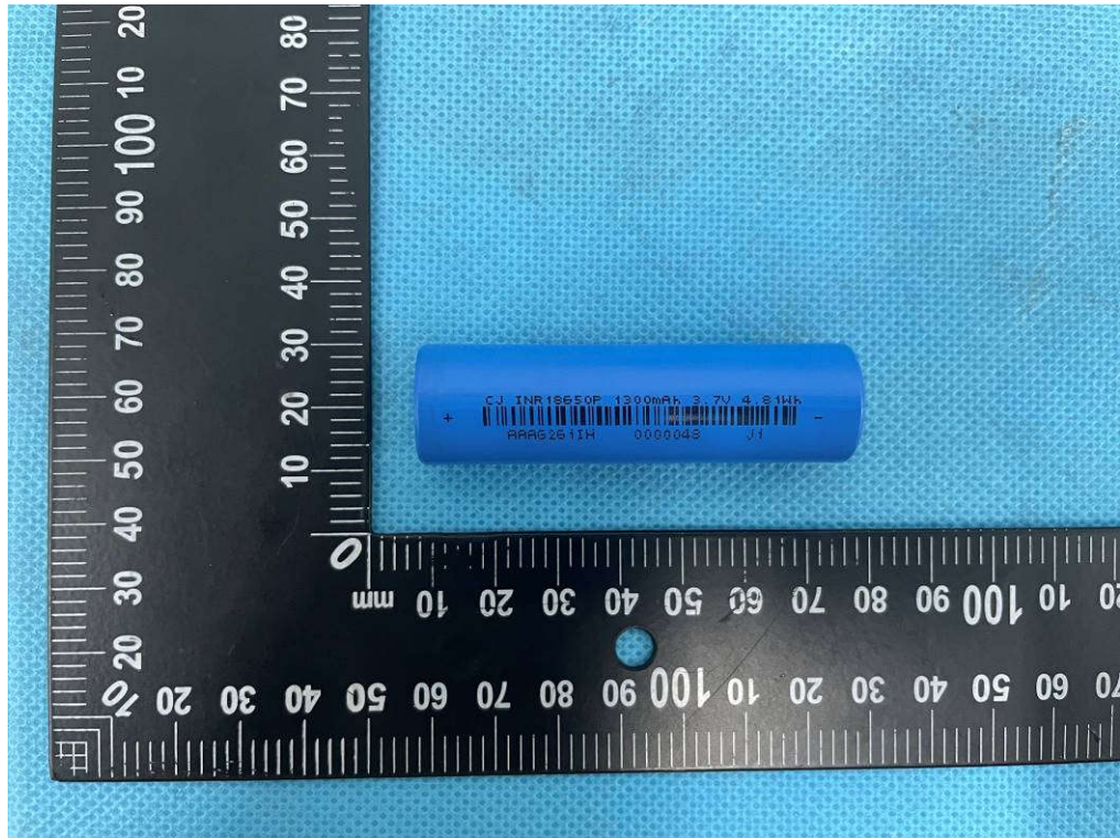
Figure 3 Front view of cell (Model: INR 18650P-1300mAh)
