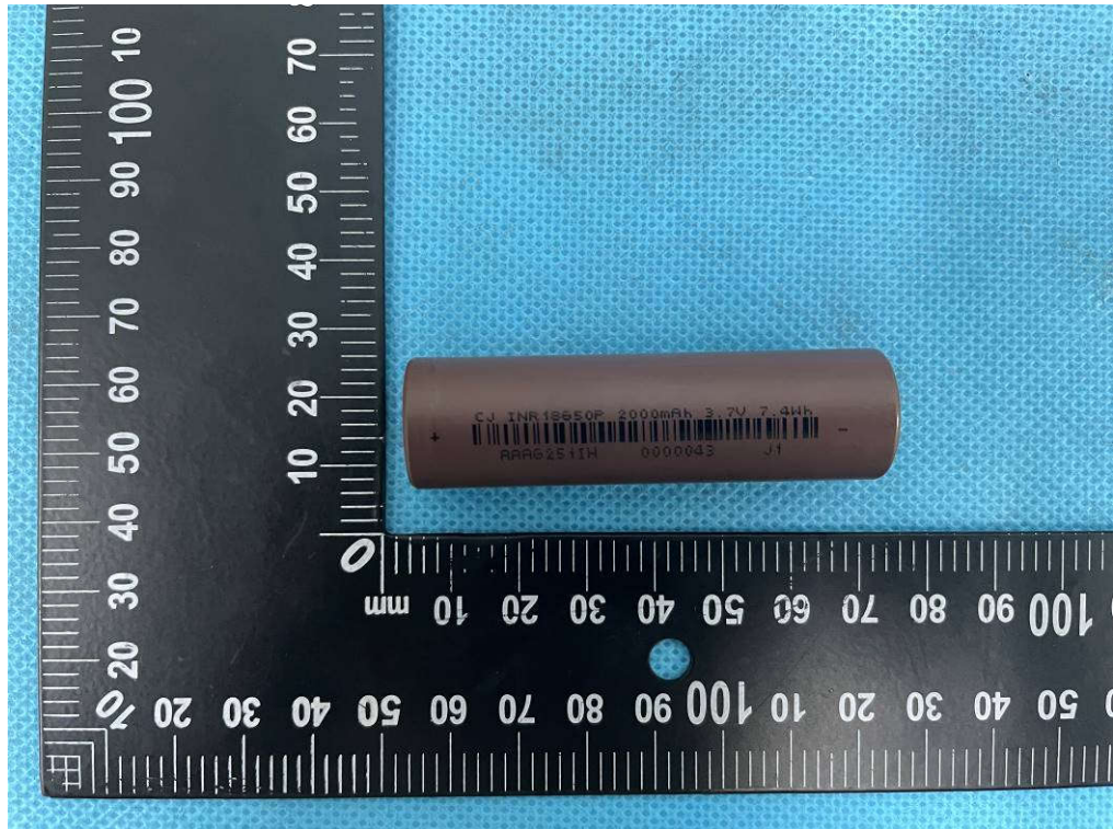
Figure 9 Front view of cell (Model: INR 18650P-2000mAh)
