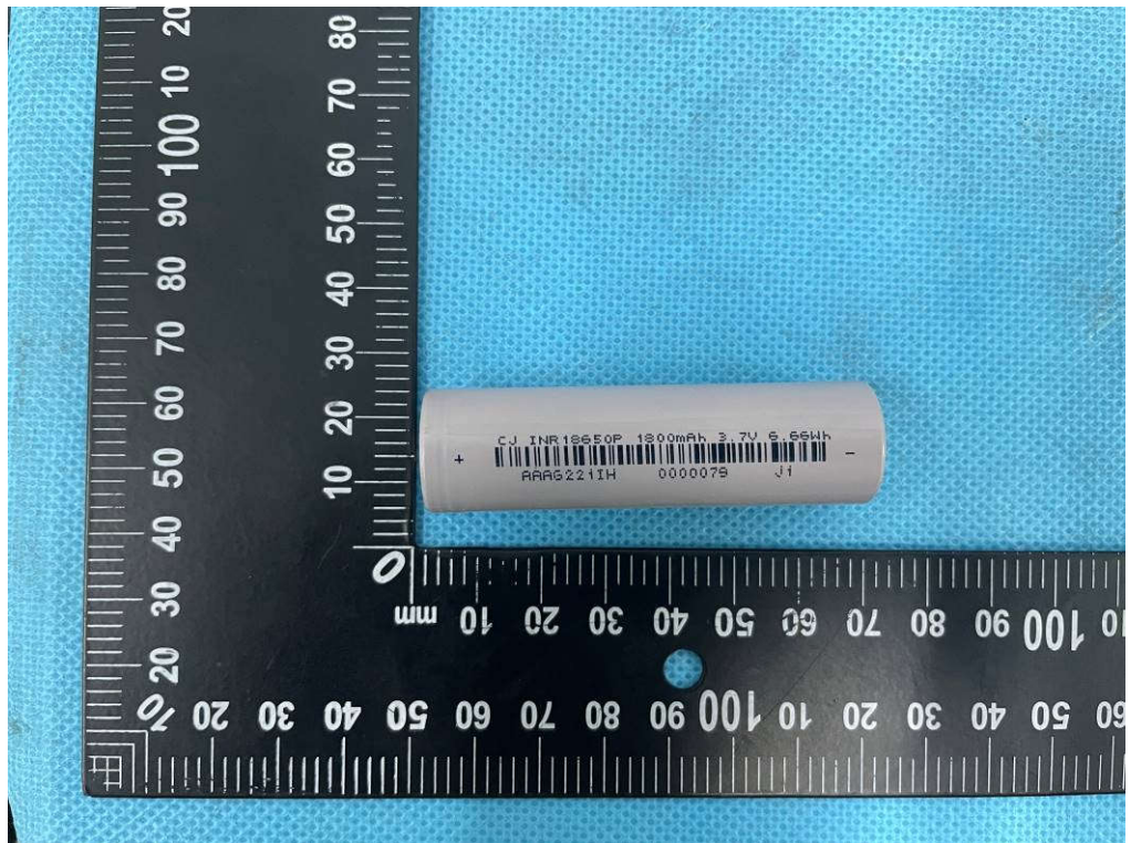
Figure 7 Front view of cell (Model: INR 18650P-1800mAh)
