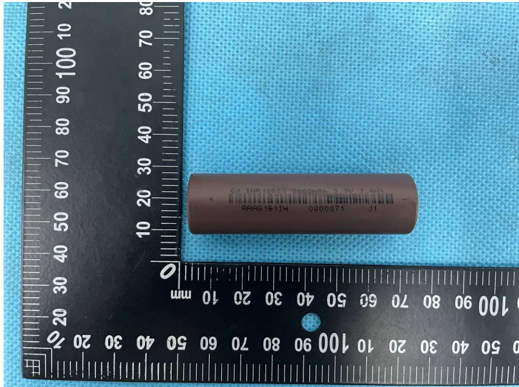
Figure 15 Front view of cell (Model: INR 18650-2000mAh)
