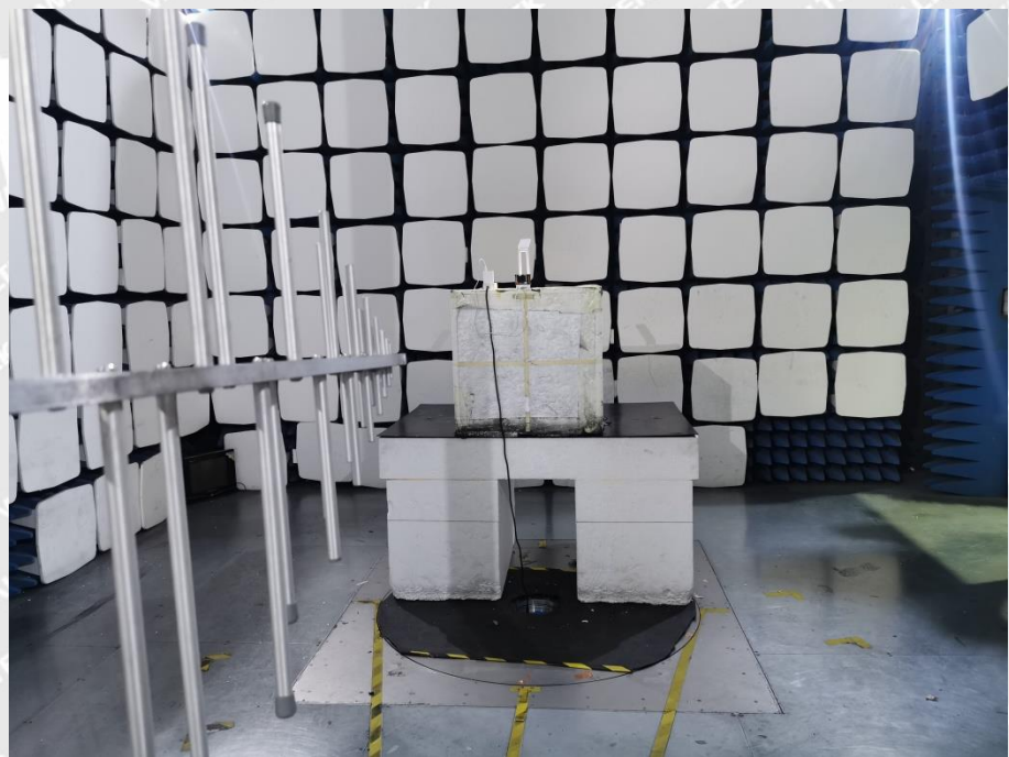
Radiated Spurious Emission Test Setup (Above 30MHz)
