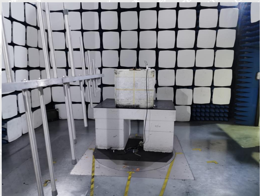
Radiated Spurious Emission Test Setup (Above 30MHz)
