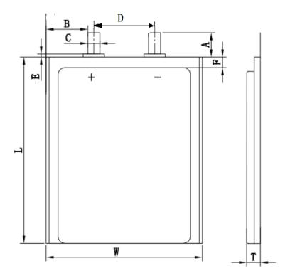
T(Max.): W(Max.): L(Max.) = 12.0mm: 60.0mm: 90.0mm
