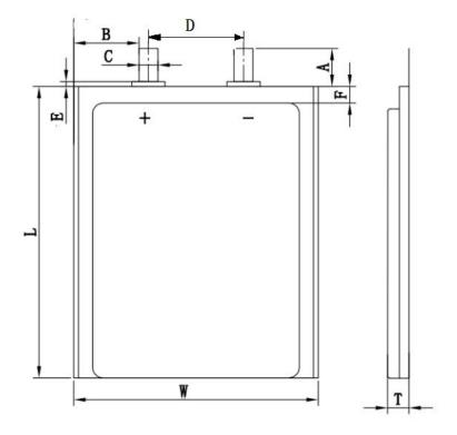
T(max.): W(max.): L(max.)=6.5mm: 60.5mm: 90.5mm
