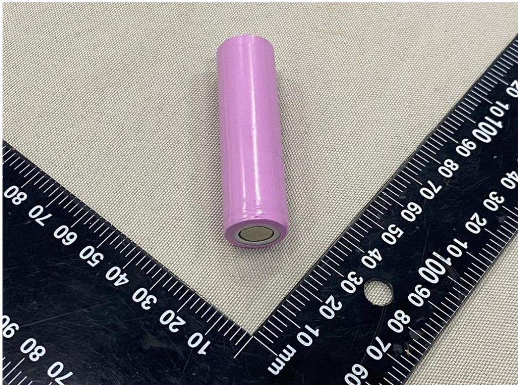
Figure 2 Side view of cell (IMR18650-3000mAh)
