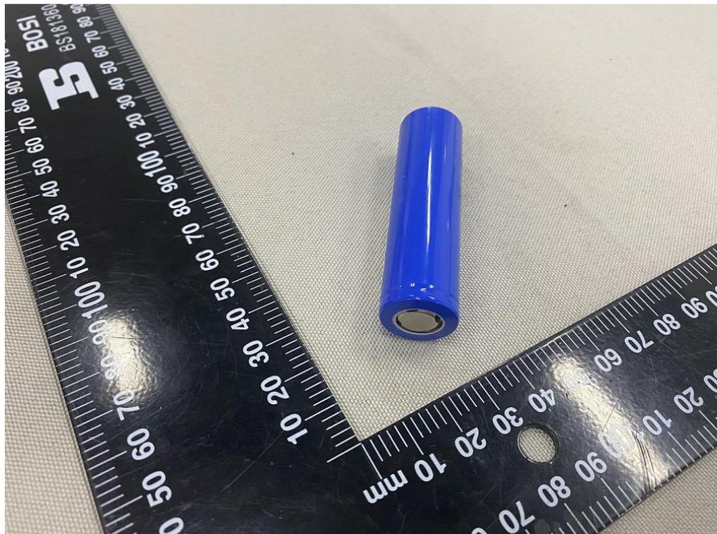
Figure 18 Side view of cell (IMR18650-800mAh)
