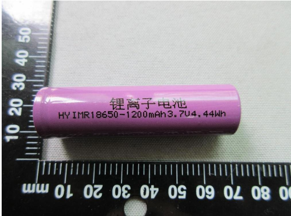
Figure 15 Front view of cell (IMR18650-1200mAh)
