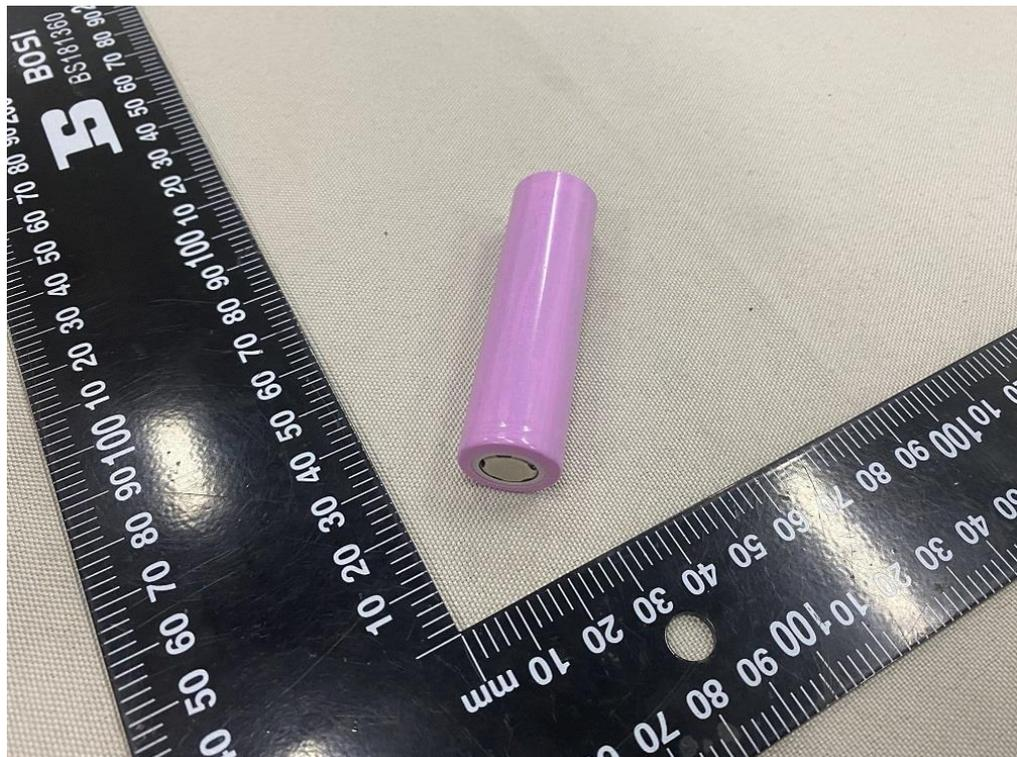
Figure 8 Side view of cell (IMR18650-2200mAh)
