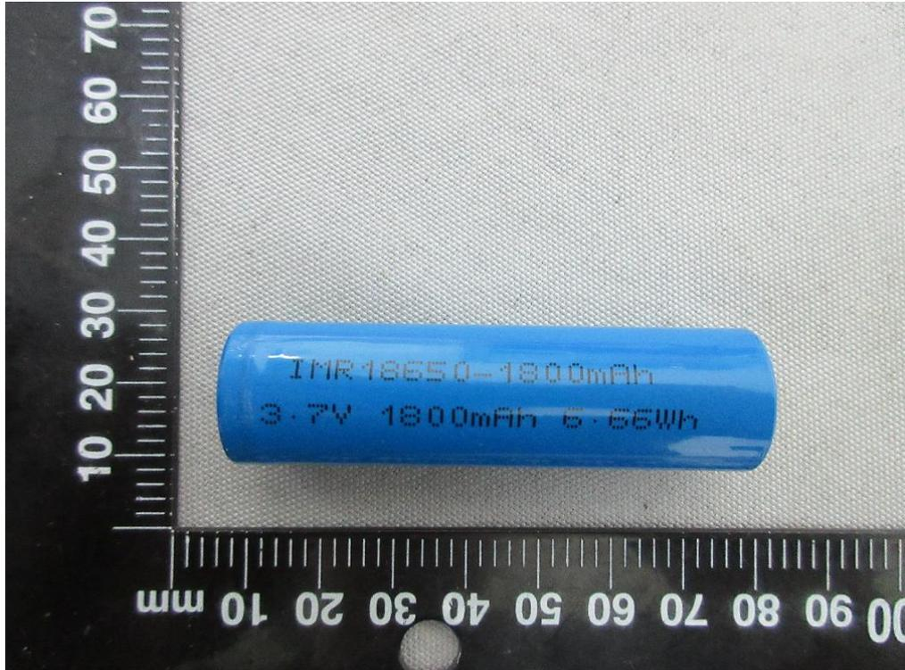
Figure 11 Front view of cell (IMR18650-1800mAh)
