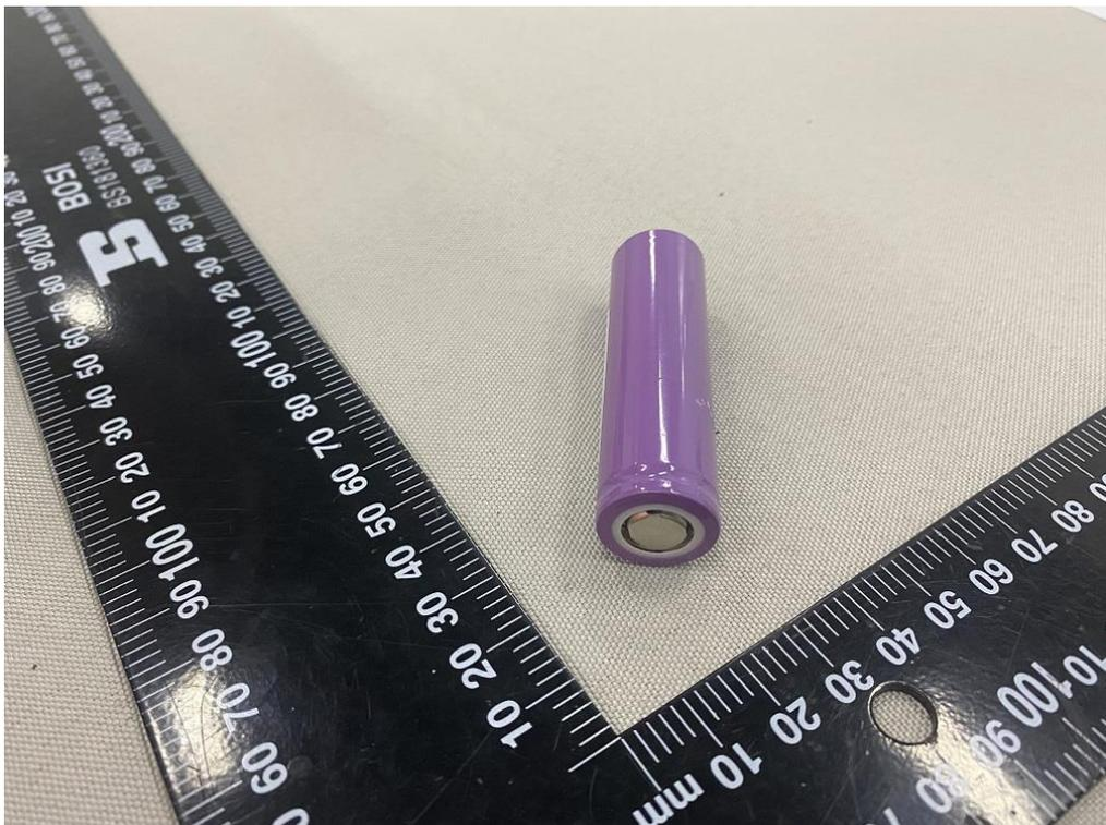
Figure 16 Side view of cell (IMR18650-1200mAh)
