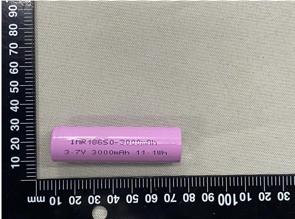
Figure 1 Front view of cell (IMR18650-3000mAh)
