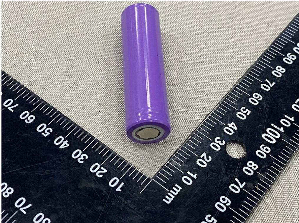
Figure 10 Side view of cell (IMR18650-2000mAh)
