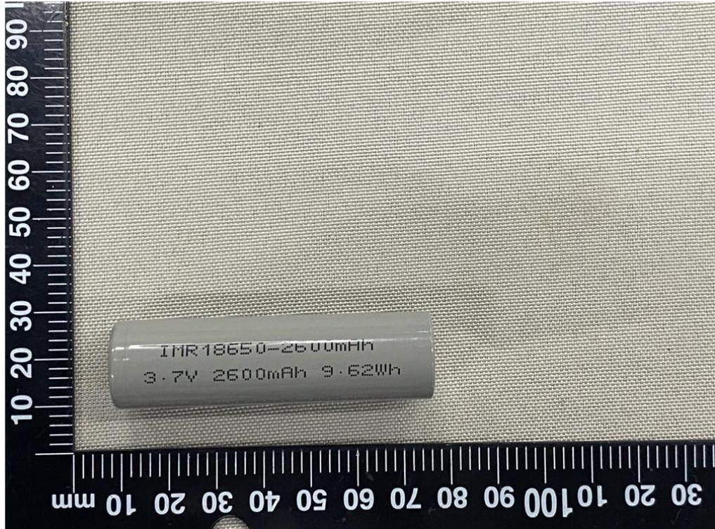
Figure 3 Front view of cell (IMR18650-2600mAh)
