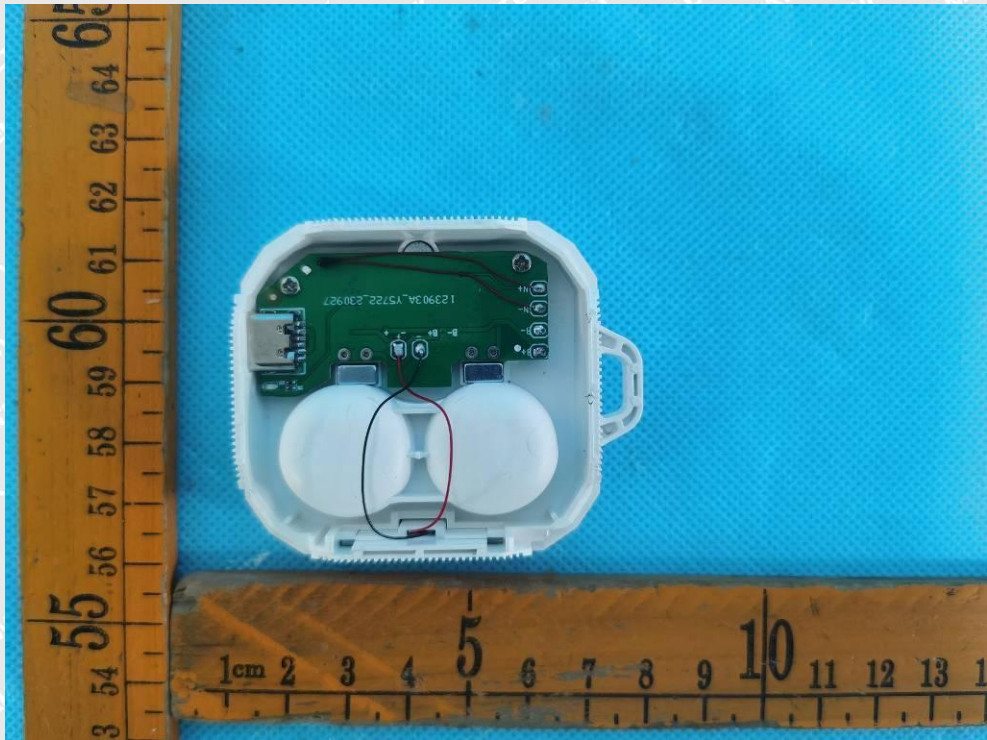
Figure 7: Internal view for charging base
