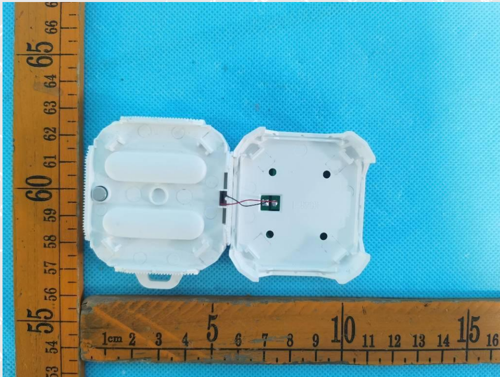
Figure 9: Internal view for charging base
