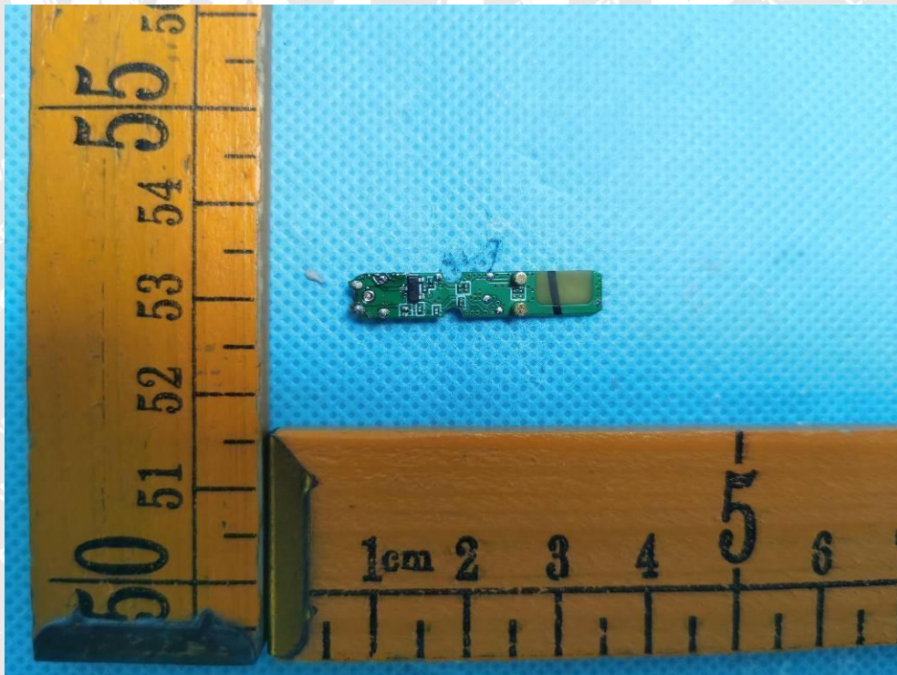
Figure 18: PCB view for earbuds
