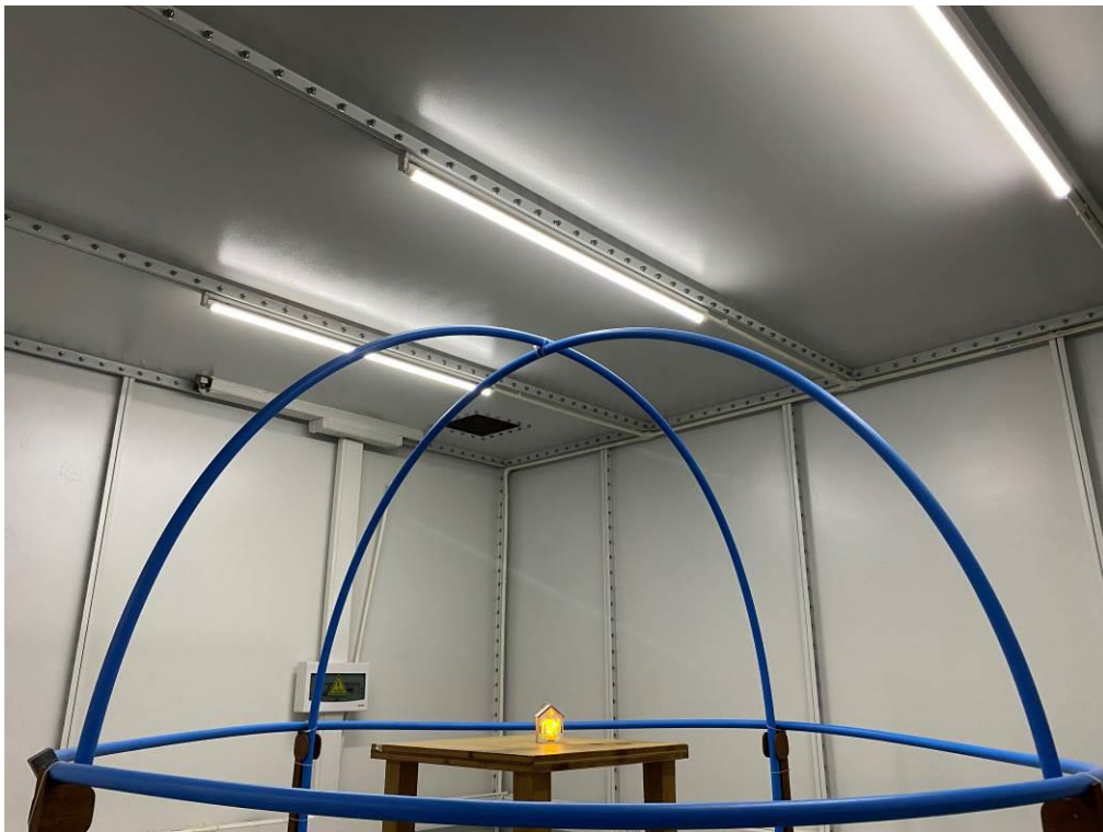
EN IEC 55015 RADIATED ELECTROMAGNETIC DISTURBANCE TEST SETUP
